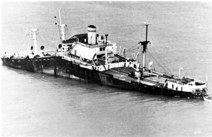
The vessel the ELENI K lying with a broken back.
