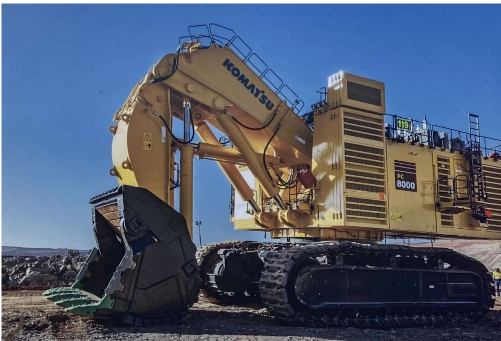
Super Pit Face Shovel Bucket. The bucket weighs 68 tonnes, the size is 38 cubic metres, and the cost is $1.1 million. I hate to think what the machine the bucket is attached to costs.
